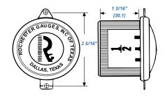
Note: This dial is used in conjunction with 93-2 mounting bracket and 39-2 bezel.
