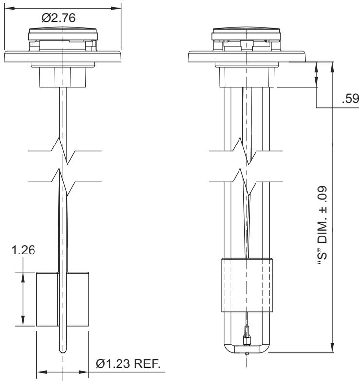
The Rochester magnetic liquid level gauge operates simply by means of a float actuating a powerful magnet inside the container which in turn provides an invisible “magnetic coupling”, through a solid head, with the magnet on the pointer in the dial chamber. Thus the gauge head completely seals off the liquid in the container so the dial may be removed and replaced quickly anytime without loss of liquid.
