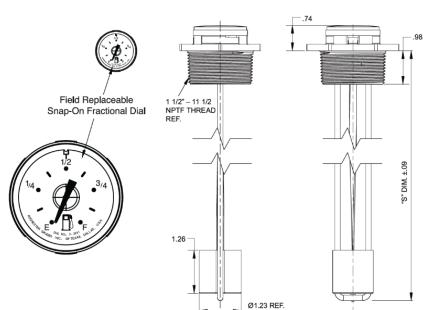
The Rochester magnetic liquid level gauge operates simply by means of a float actuating a powerful magnet inside the container which in turn provides an invisible "magnetic coupling", through a solid head, with the magnet on the pointer in the dial chamber. Thus the gauge head completely seals off the liquid in the container so the dial may be removed and replaced quickly anytime without loss of liquid or vapor.
