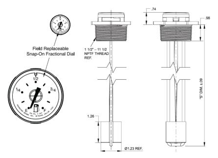
The Rochester magnetic liquid level gauge operates simply by means of a float actuating a powerful magnet inside the container which in turn provides an invisible "magnetic coupling", through a solid head, with the magnet on the pointer in the dial chamber. Thus the gauge head completely seals off the liquid in the container so the dial may be removed and replaced quickly anytime without loss of liquid or vapor.
