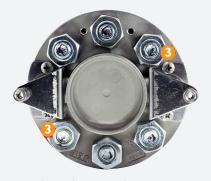
Note: For 8" dials remove all three existing brackets attached to the head and install two 4" dial brackets (0093s00001; sold separately) with 2 screws (0040-00413) each bracket. You may use 4 of the 6 screws from removal of existing dial brackets for 8" dial.
