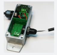
4. Pull cable through the water-proof fitting, once the cable's jacket is past the rubber gasket. Tighten the glands cover to close the seal to 22 lbf·in (2.5 N·m). Attach the wires to the terminal block, pay close attention to polarity.
