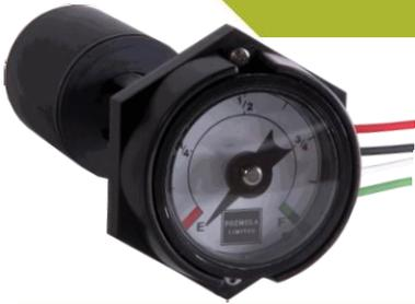
The **G/LL65** vertical spiral gauge is a mechanically operated liquid level gauge with a local display and two electrical outputs. Suitable for connection to a typical controller or remote level indicator the outputs are; a variable resistance proportionate to the liquid level and a volt-free switch to trigger an alarm when the liquid reaches a prescribed level. To avoid a potential leak path, the gauge features a magnetic coupling between the float driven spiral and the level indicator.
