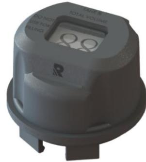
The 6318 Wireless BLE Dial provides a wireless reading of a Rochester Mechanical Gauge installed in a tank. The unit replaces the existing snap-on or screw-on dial and optional wired R3D module with a new BLE Dial that broadcasts tank volume over Bluetooth. An integrated LCD display shows the tank volume as a percentage.
