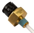
The **S281** is an active device designed to give an alarm signal if coolant falls below, or rises above, a preset level. It can be specified with a delay to eliminate false alarms due to turbulence.
