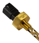
The **S284** is an active device designed to give an alarm signal if liquid falls below, or rises above, a preset level. It can be specified with a delay to eliminate false alarms due to turbulence.
