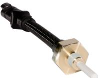
The **5287** is an active device designed to give an alarm signal if liquid falls below, or rises above, a preset level. It can be specified with a delay to eliminate false alarms due to turbulence and the flying lead enables customers to specify a suitable connector of their choice.
