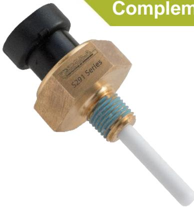
The **S291** is an active device designed to give an alarm signal if liquid falls below, or rises above, a preset level. It can be specified with a delay to eliminate false alarms due to turbulence.
